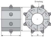
With standard dies. Crimping range can be increased with special dies.
